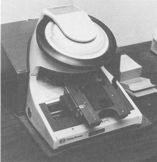
FIG. 8—Foot-activated electric embosser for preparing plastic plates to imprint labels.
